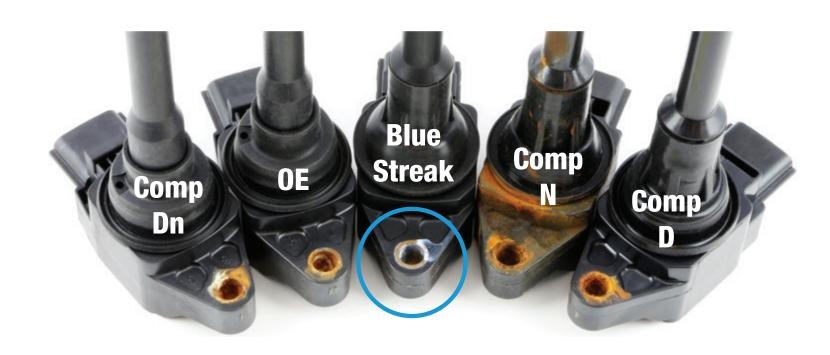
Blue Streak® UF549 has an upgraded brass bushing which outperformed the OE and competitors in a 200-hour salt spray test.
