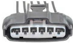
S2817 Accelerator Pedal, Electronic Throttle Body Hyundai, Infinity, Lexus, Nissan, Scion, Subaru, Toyota (2019-2001)
