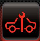
**Service Vehicle Soon:** Typically indicates a lighting or other electrical problem that is controlled by the BCM (body control module). Check all lights, headlights, turn signals, brake lights, and hazard lights. This symbol may also warn driver of a traction control problem, or a communication problem between modules.
