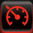
**Cruise Control:** Indicates that the cruise control system is engaged while the vehicle is driving.
