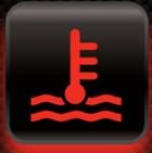
**Coolant Temp Warning:** Indicates temperature has exceeded normal limits. Check coolant level, fan operation, radiator cap, and coolant leaks.
