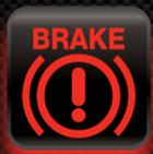
**Brake System:** Indicates one of three possible conditions: parking brake is on; problem with the braking system/brake fluid is low; or ABS problem. Check brake fluid; make sure parking brake is fully released. If this is an ABS system, problem may need a professional diagnosis.
