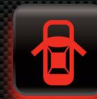
**Door Ajar:** Indicates a door (including hood and trunk) is not closed. Open and close all doors, including hood and trunk. If vehicle is left in this condition overnight, it can drain the battery.
