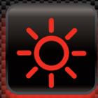
**Lamp Out:** Indicates that there is an exterior light on the vehicle that is not functioning properly.
