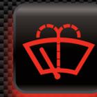
**Washer Fluid Reminder:** Indicates washer fluid is low. Fill washer fluid reservoir. The cap has a symbol that looks like a windshield. Some vehicles have separate reservoirs for front and rear window washers.
