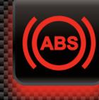
**ABS Light:** Indicates that the Anti-lock Brake computer has set a code and needs professional diagnosis.
