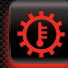
**Transmission Temperature:** Transmission is operating at higher than optimum temperature as transmission fluid is hotter than normal. Check transmission fluid level and engine coolant level.
