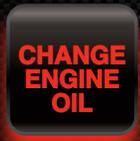
**Oil Change Reminder:** Indicates that oil life has expired. This is monitored by the ECM; the interval can be mileage or a combination of readings taken by the ECM. The reset procedure is listed in the owner's manual. Some vehicles require the use of special tools to reset the light.
