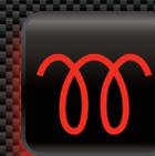
**Glow Plug (Diesel):** On diesel vehicles this light indicates that the engine's glow plugs are warming up and the engine should not be started until light goes out.
