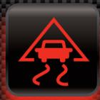
**Traction Control or ESP:** Illuminates when the vehicle's traction control/anti-skid or electronic stability system is in use. Usually an indicator that conditions are slippery.
