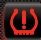
**TPMS (Tire Pressure Monitoring System):** Indicates the tire pressure monitoring system has found a tire with low air pressure or a sensor with a dead battery or malfunction. Check tire pressure. Some vehicles will allow manual reset of TPMS light and others will require professional diagnosis. Refer to owner's manual.
