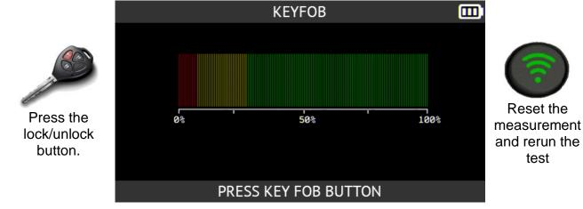
The tool will wait for a signal and then display the strength of the signal it receives.
